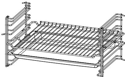
You can use the tray as a drip tray for grilled food and meat dishes by placing the tray and the rack together.
