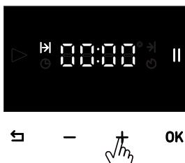
Firstly, select the minute with -/+ buttons and activate the clock by pressing on OK button.
