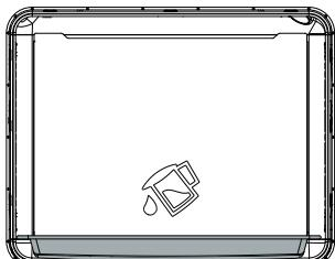
The dirt can be wiped easily by softening them after cooking. Remove all the accessories (if there is a wire rack) from the oven. Place the single tray on the lowest base by adding some water in it and by selecting Lower Heating function ,  operate the oven at for 100°/20 minutes. At the end of the operation, wipe the inside of the oven with a damp cloth or sponge.
