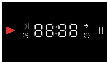
It is an electronic timer which makes the food to be cooked prepared at the time you desire. You should adjust the cooking duration of the meal and the time when you desire it to be prepared.
