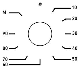
It allows you to set the time for the food to be cooked. You can set it by selecting the temperature and type of cooking, turning the cooking time clockwise. When the time is up, it warns with a ringing sound. If you wish, you can start cooking by selecting the temperature and type of cooking without selecting a time by setting it to M mode.
