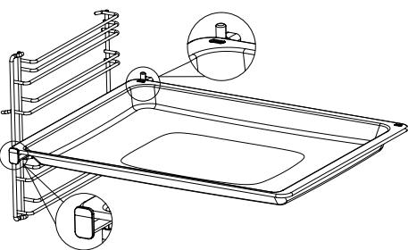
Push the rails completely inside without placing the tray and wire grid on them. Accessories must be between the front and rear overhangs of the rails.
